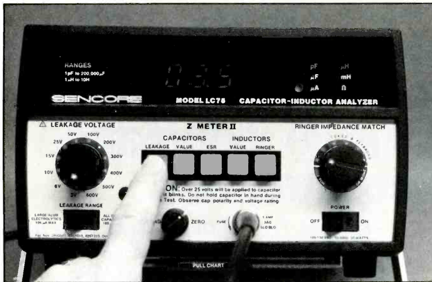
This capacitor-leakage test showed low leakage, but at a low 6V. If the capacitor voltage rating is between the LC-75 voltages, use the next lowest.
